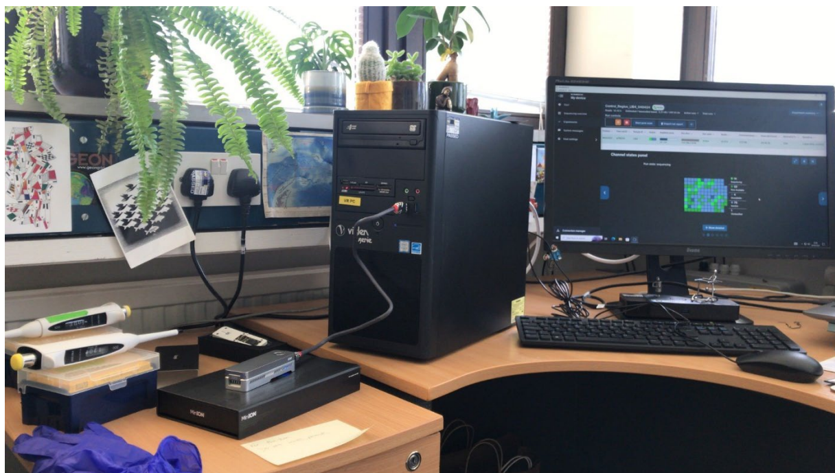
Figure 1: Set up for the sequencing of the first library of the control region samples, showing the MinIon device connected and running the experiment.
